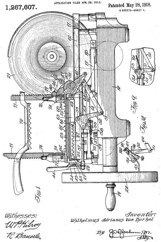
W. A. VAN BERKEL. SLICING MACHINE. APPLICATION FILED APR. 28, 1913.
